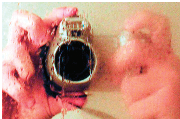
Figure 5. Mirror glass coated with acrylic acid copolymer on the left and uncoated glass on the right exposed to saturated water vapor environment.
